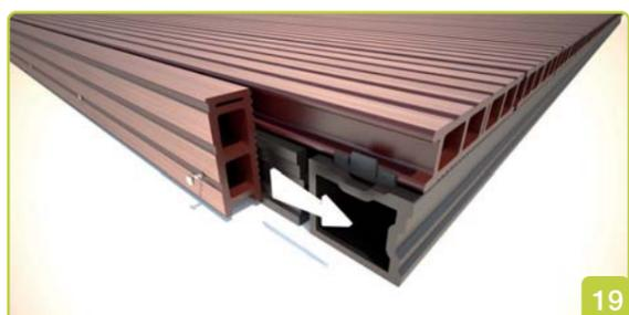
Fixing the Edenex Plank as a skirting board is relatively simple. Screw through the plank, into the Edenex plank edge with no more than 500mm between fixings using screws long enough to engage the second rib on the deck plank. Fig 19.
