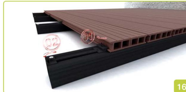
To fix the final plank, simply screw the end clip into position using the previous centre clip as a locator (Fig 16). Repeat the action of engaging the plank in the centre clip, then push the board into position, making sure that the end clip locks the final plank in place as you did for the first plank (Fig 9).
