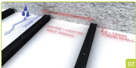
Once the completed support framework has been laid and secured, you can begin installation of the Edenex Planks. Cut the planks to length using a power saw with fine tooth carbide blade allowing for the expansion gaps mentioned above. Make allowance for expansion in length of 3mm per metre length on all planks and 3mm in width in each plank.
