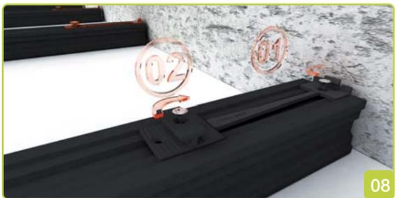
Starting at the top, place the End Clip into the groove on the Support Beam and secure in place ensuring that the end of the clip with the screw hole is flush with the edge of the support beam as shown in Fig. 8 - 1.
