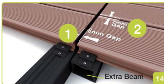
When placing planks end to end it is important to allow a minimum of 8mm between planks. This distance will slowly close as the planks expand. (Fig 14-1).
