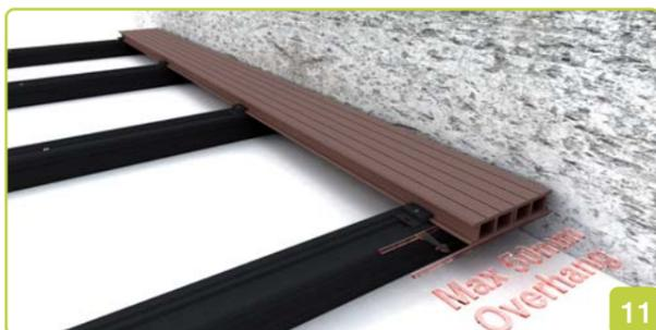
If the Edenex plank finishes parallel to a wall or structure, it is essential to leave a gap between the plank and the wall. Allow a 4mm gap along the length and a 10mm gap at the end (Fig 12).
