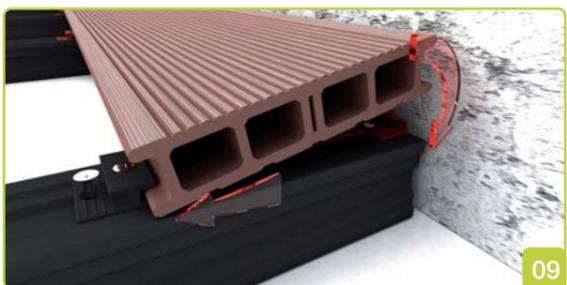
Position the decking plank, so that it fully engages in the fixed Centre Clip. Then, push the decking plank downwards as shown in Fig 9. This will engage the clip action of the end clip, and the plank will lock into position.
